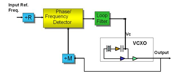
A typical PLL application using a VCXO is depicted in Figure 1. In this application the designer must make sure the PLL remains locked under all conditions including the life time of the product.
