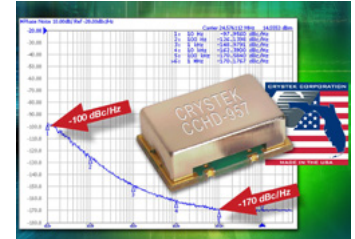
The CCHD-957 from Crystek has a typical noise floor of -170 dBc/Hz @ 100kHz offset.
