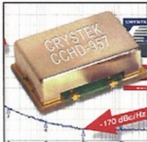
SMT crystal clock oscillator.
