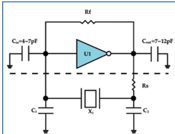
Figure 3: Pierce-Gate Showing Internal Input and Output Capacitances
